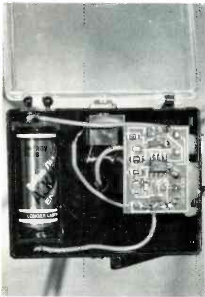
FIG. 3—THE COMPLETE SMT AMPLIFIER, including an N-battery and an earphone jack, can be assembled in a small plastic pill box.
