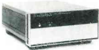
FIG. 7—THE HP 59301A ASCII-to-parallel converter accepts byte-serial ASCII characters from the GPIB, then converts them to parallel output.
